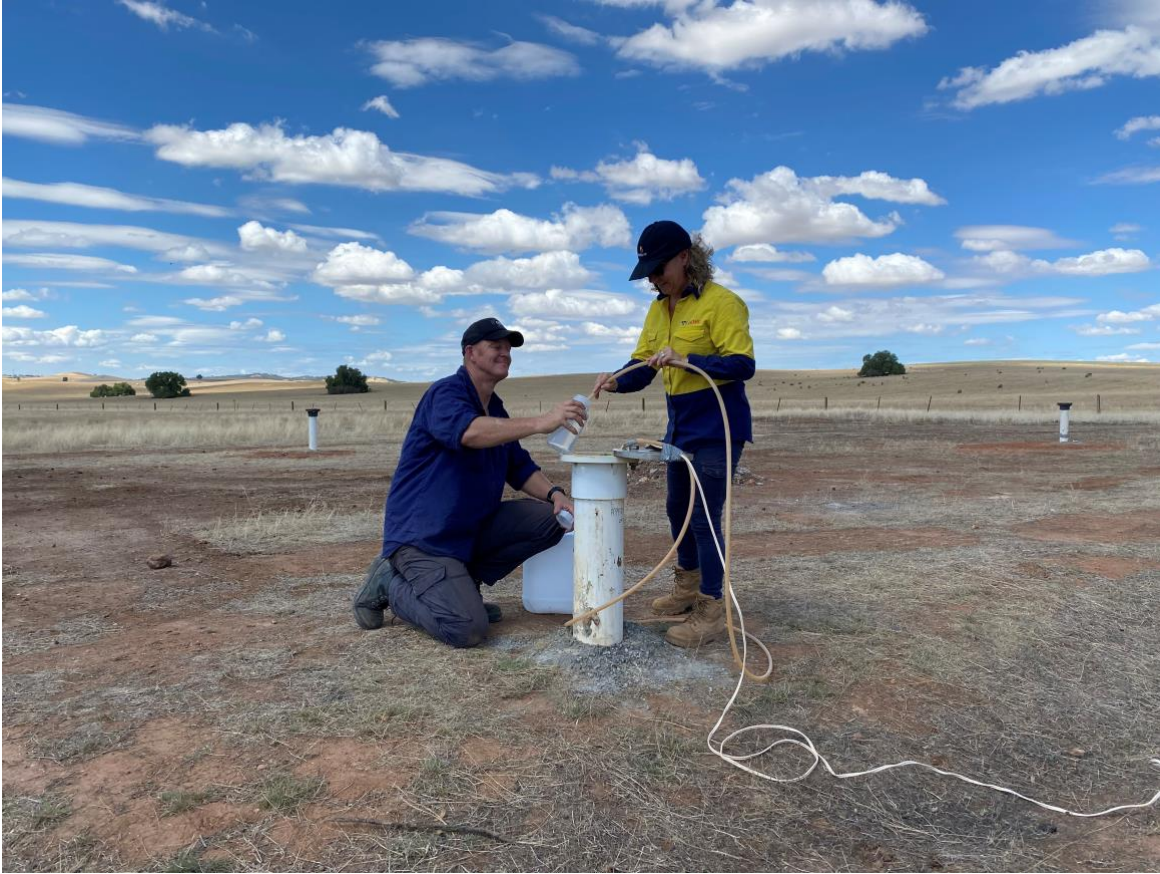
Photo 4: Push-Pull Tracer Trials Underway at Kapunda
