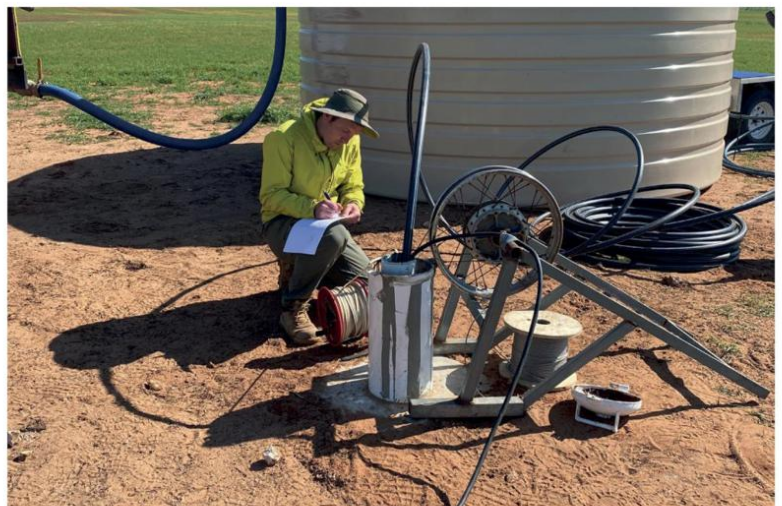
Figure 3. Hydrogeologist carrying out pump test.
